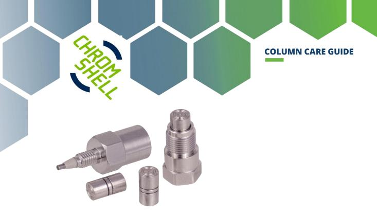
Protection can be perfectly ensured by installing a pre-column filter holder with a  $0.2\mu m$  or  $0.5\mu m$  frit. This in-line filter can withstand pressures of up to 1375 bars and is easy to use. The filter holder consists of a two--piece body and replaceable filter – a metal frit.
