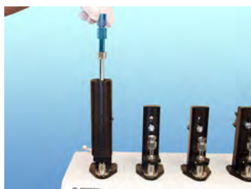
4 Insert tube with fitting into tube heater.
