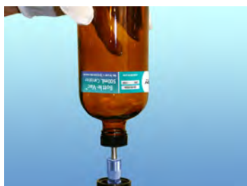
6 Attach an evacuated container to the top.
